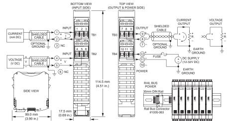
Multi-range ±20mA or ±500mV input ◆ Universal current/voltage output ◆ 12-32V DC local/bus power
