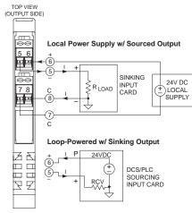
Potentiometer/slidewire, thermistor input ◆ 4-20mA output (sink/source) ◆ 12-32V DC loop/local power
